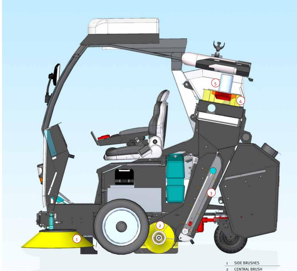
3 CONVEYOR BELT4 DUST FILTER5 SUCTION TURBINE
