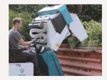
**HIGH DUMP** The robust hydraulic system allows to raise the whole collection group and unload directly into a container.
