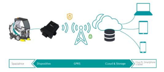
A telematic device is installed on board the sweeper that allows you to:
